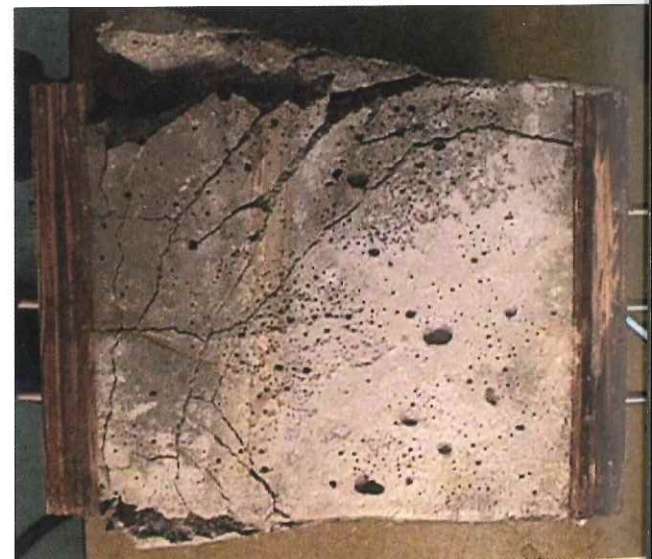
Fig. 1: The bottom of a mortar bar exposed, at the top, to a 35% calcium chloride brine for 2 months at 23^\circ\text{C} ( 73^\circ\text{F} ) (photo courtesy of A. Poursaee and C.M. Hansson)
