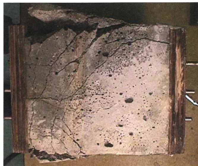
Fig. 1: The bottom of a mortar bar exposed, at the top, to a 35% calcium chloride brine for 2 months at 23°C (73°F) (photo courtesy of A. Poursaee and C.M. Hansson)
